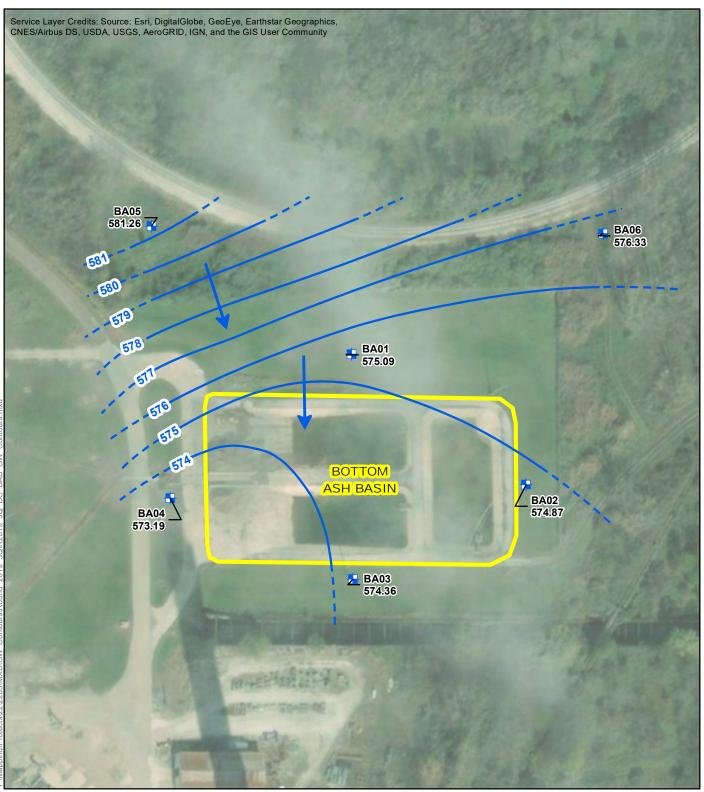
CCR RULE MONITORING WELL DUCK CREEK BOTTOM ASH BASIN (UNIT ID: 205) ÷ LOCATION **GROUNDWATER ELEVATION CONTOUR MAP** GROUNDWATER ELEVATION CONTOUR (1-FT CONTOUR INTERVAL, NAVD88) INFERRED GROUNDWATER CCR RULE GROUNDWATER MONITORING ELEVATION CONTOUR DUCK CREEK POWER STATION GROUNDWATER FLOW CANTON, ILLINOIS DIRECTION CCR MONITORED UNIT
